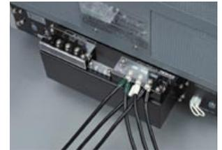
▲When two PT01-PCR-LA terminals are connected
