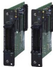
This option allows the PCR-LA Series system to be used as a single-phase, three-wire power supply.
