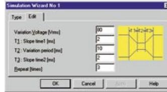
(Left) Wizard for abrupt phase shift simulation in single-phase output
