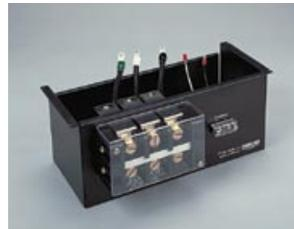
The parallel terminal is connected to the back panel of the master unit. Up to three PCR-LA Series systems can be connected in parallel to retrieve the output. The terminal combines multiple wires into a single bundle. Note that the parallel operation driver is not included.
